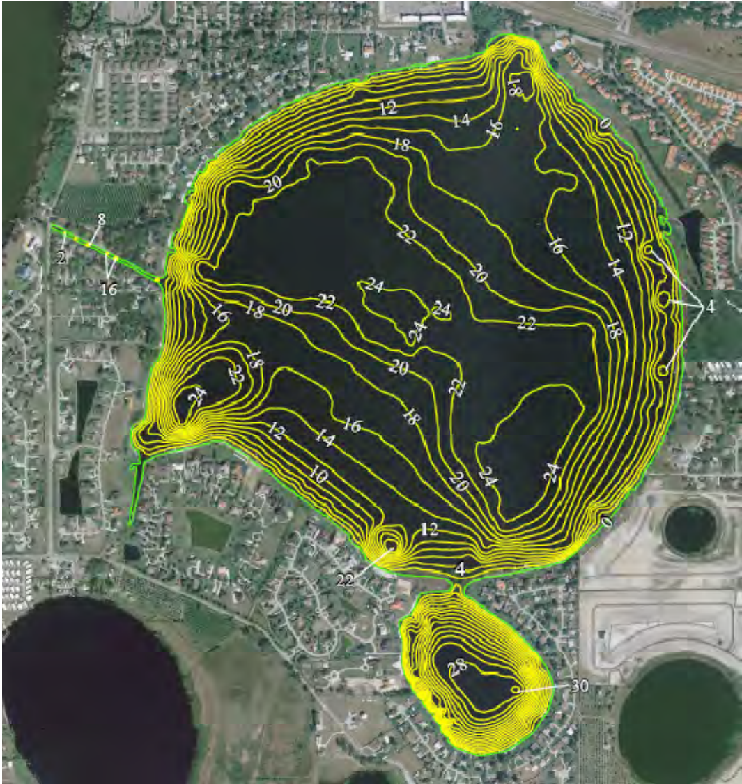
Figure 4-104. Lake Winterset bathymetry (June 2007) at water level elevation = 129 feet (Polk County Water Atlas).
