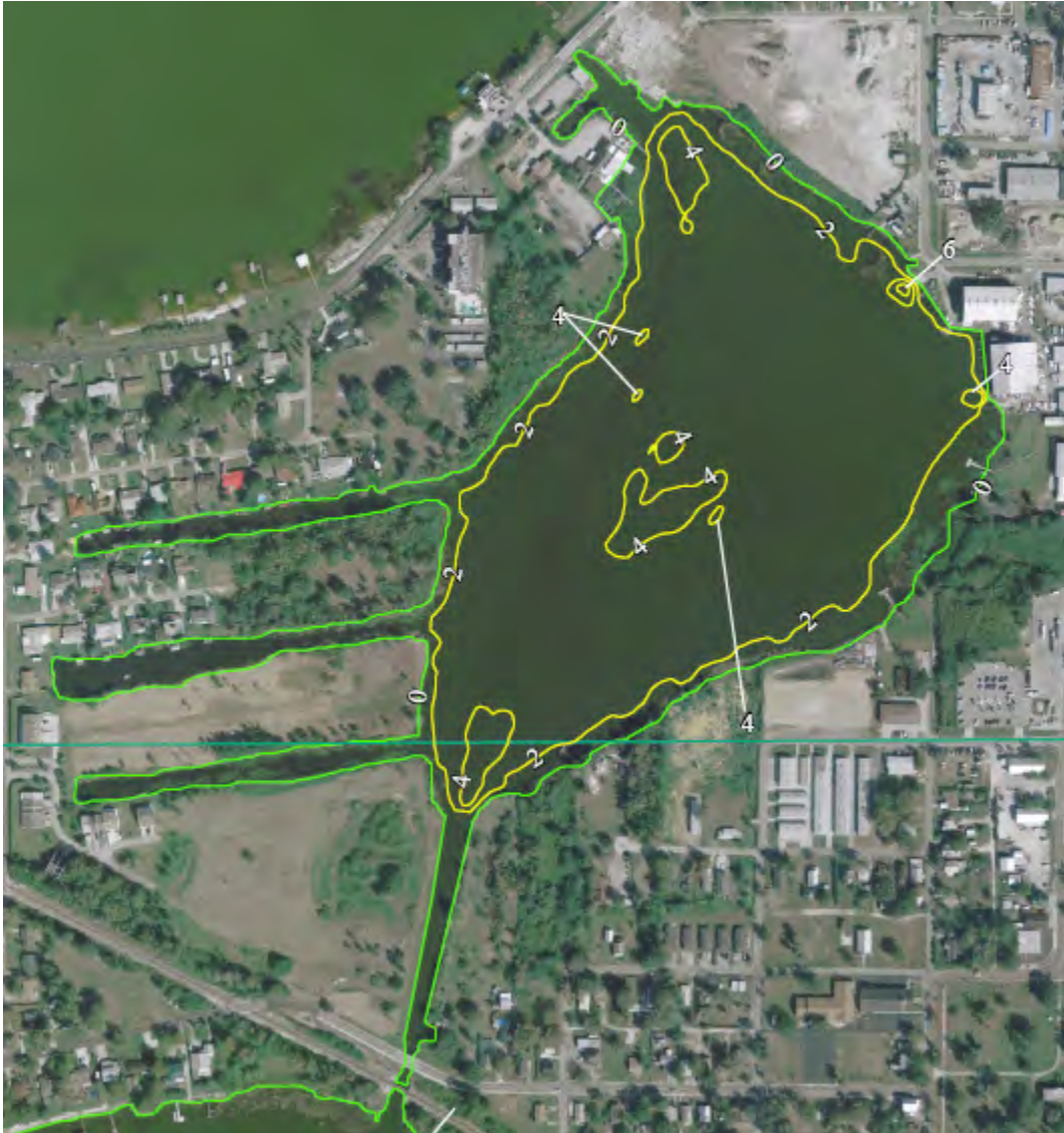
Figure 4-66. Lake May bathymetry (September 2009) at water level elevation = 130 feet (Polk County Water Atlas).
