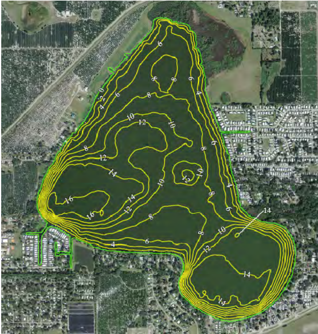
Figure 4-62. Lake Mariana bathymetry (October 2009) at water level elevation = 136 feet (Polk County Water Atlas).
