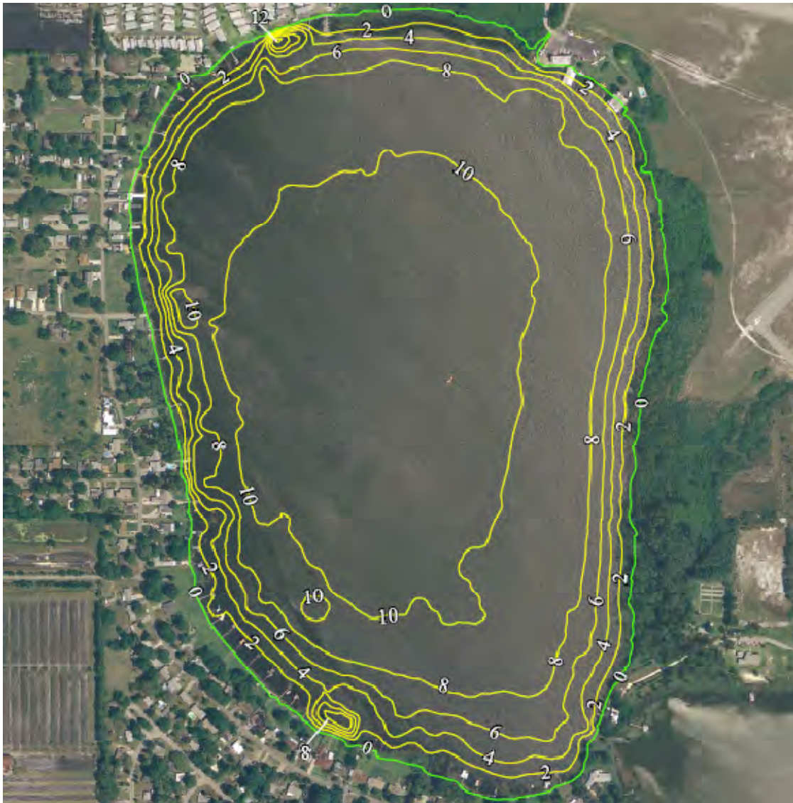
Figure 4-49. Lake Jessie bathymetry (October 2006) at water level elevation = 130 feet (Polk County Water Atlas).
