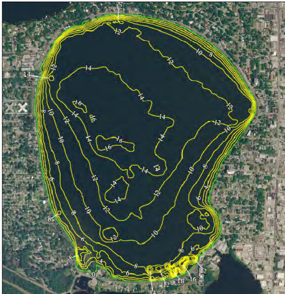
Figure 4-39. Lake Howard bathymetry (August 2005) at water level elevation = 132 feet (Polk County Water Atlas).
