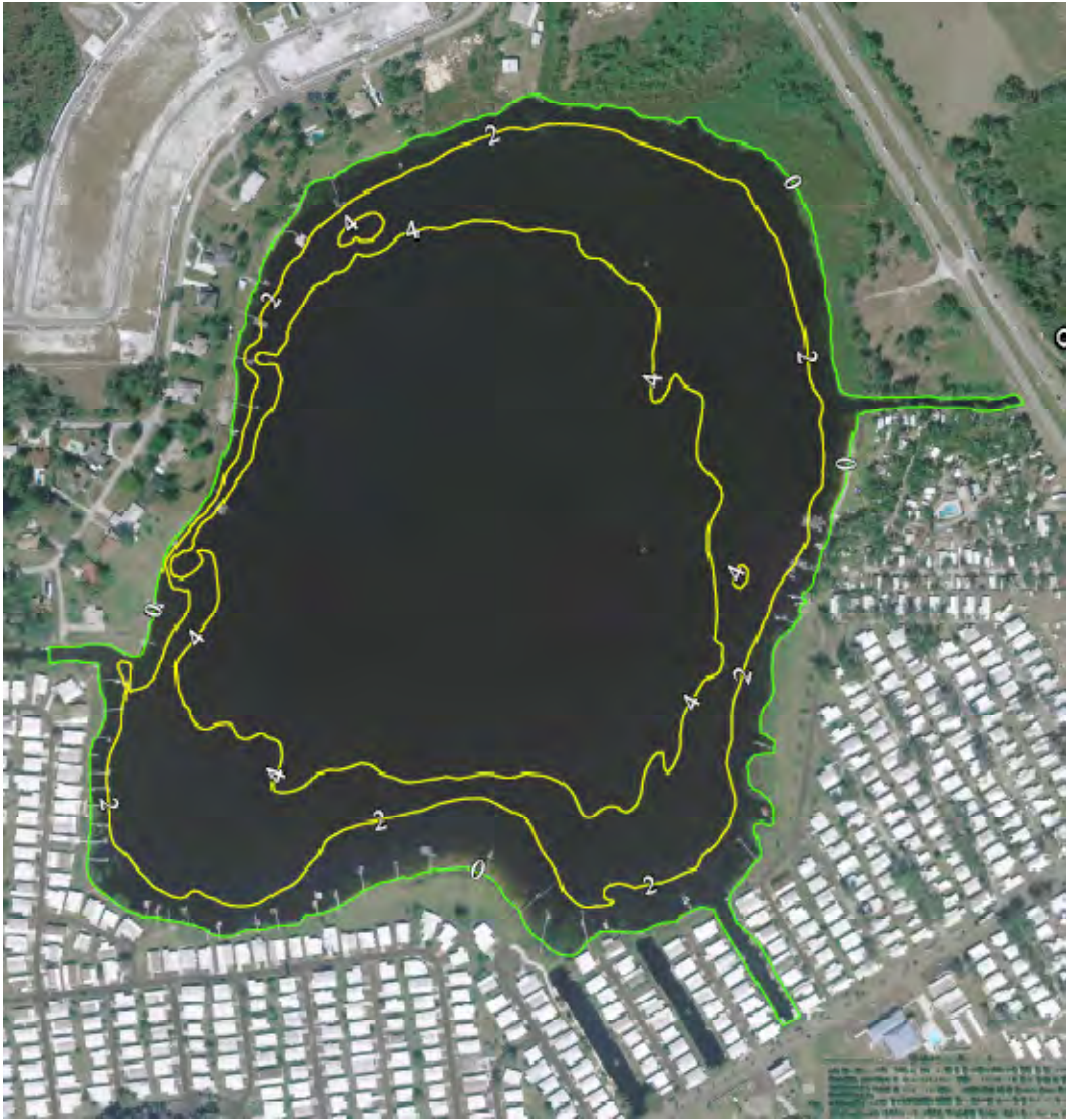
Figure 4-70. Middle Lake Hamilton bathymetry (February 2010) at water level elevation = 118 feet (Polk County Water Atlas).
