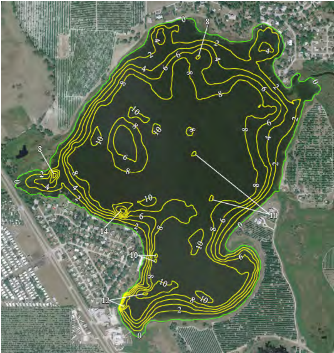
Figure 4-53. Little Lake Hamilton bathymetry (February 2010) at water level elevation = 118 feet (Polk County Water Atlas).
