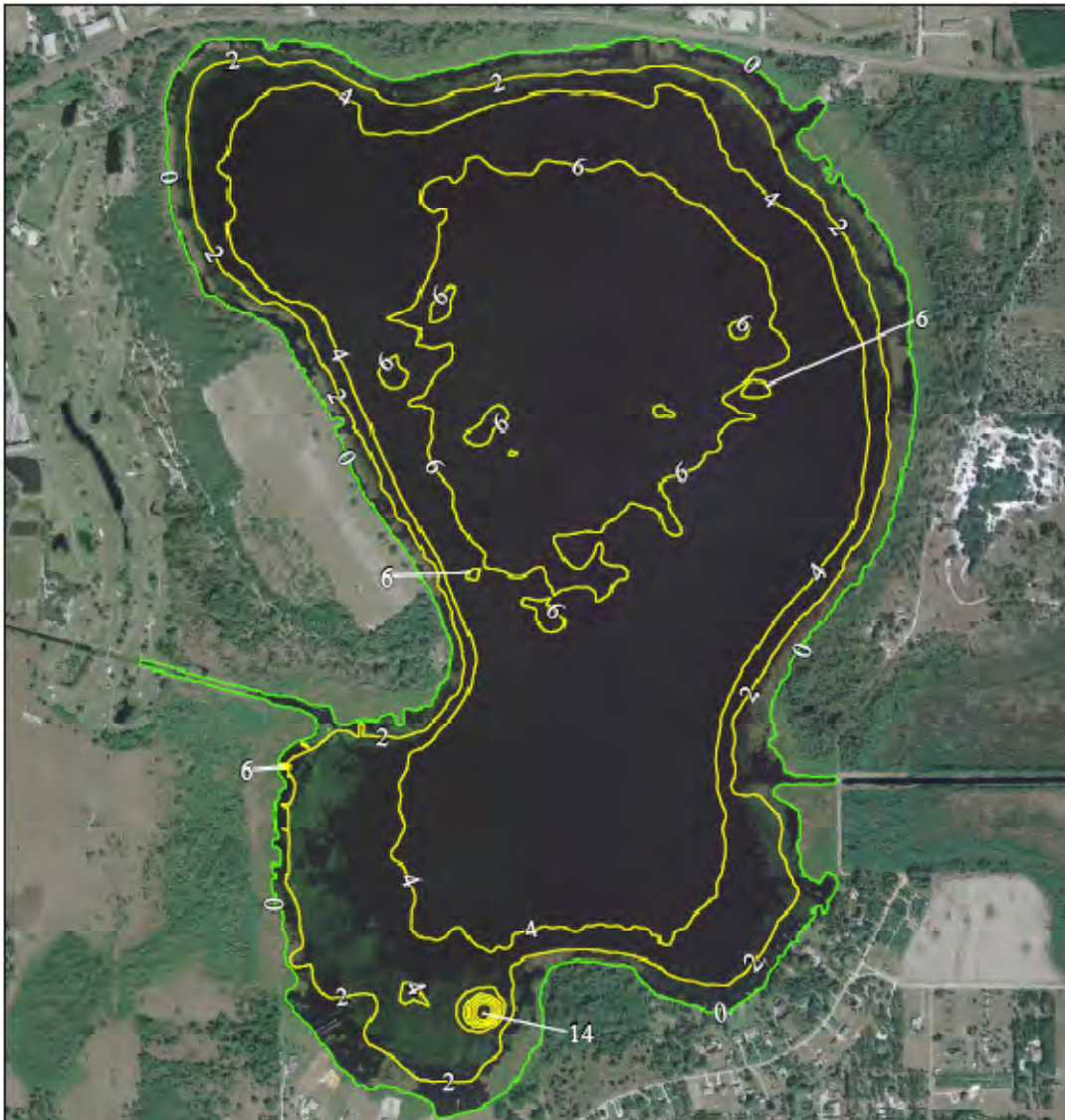
Figure 4-19. Lake Fannie bathymetry (July 2007) at water level elevation = 122 feet (Polk County Water Atlas).
