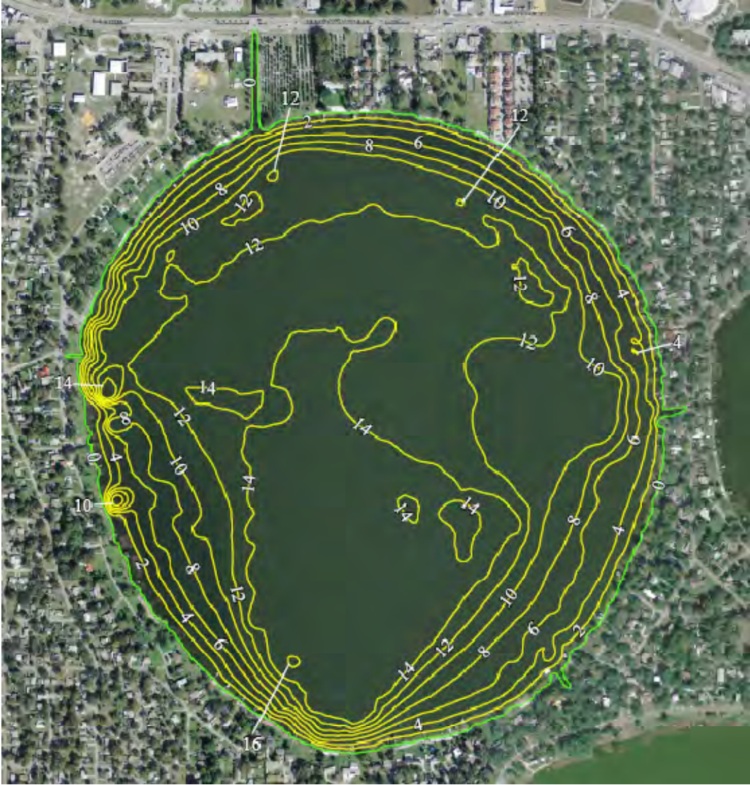
Figure 4-7. Lake Cannon bathymetry (June 2007) at water level elevation = 129 feet (Polk County Water Atlas).
