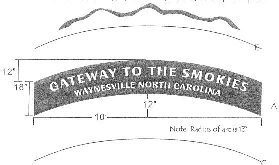
A. Identical panels, front & back. To include laser cut lettering as specified. 1/4" steel, powder coated. Panels should be assembled as single unit (Parts A, B, C, E) separate from posts. Only "D" should be permanently welded to posts. Finished project will consist of 2 identical posts and the assembled arch.
