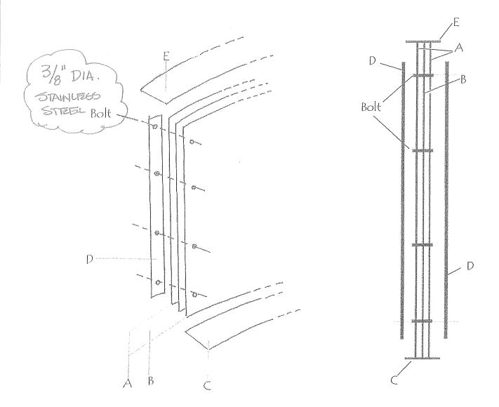
A. Identical panels, front & back. To include laser cut lettering as specified. 1/4" steel, powder coated. Panels should be assembled as single unit (Parts A, B, C, E) separate from posts. Only "D" should be permanently welded to posts. Finished project will consist of 2 identical posts and the assembled arch.
