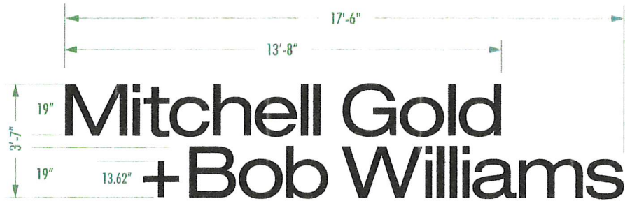
SIDE ENTRANCE SIGN ELEVATION HALO-LIT LETTERS: 3/8" = 1'-0"
