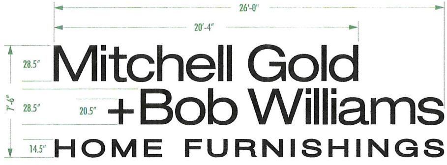
MAIN ENTRANCE SIGN ELEVATION - HALO-LIT LETTERS: 1/4" = 1'-0"
