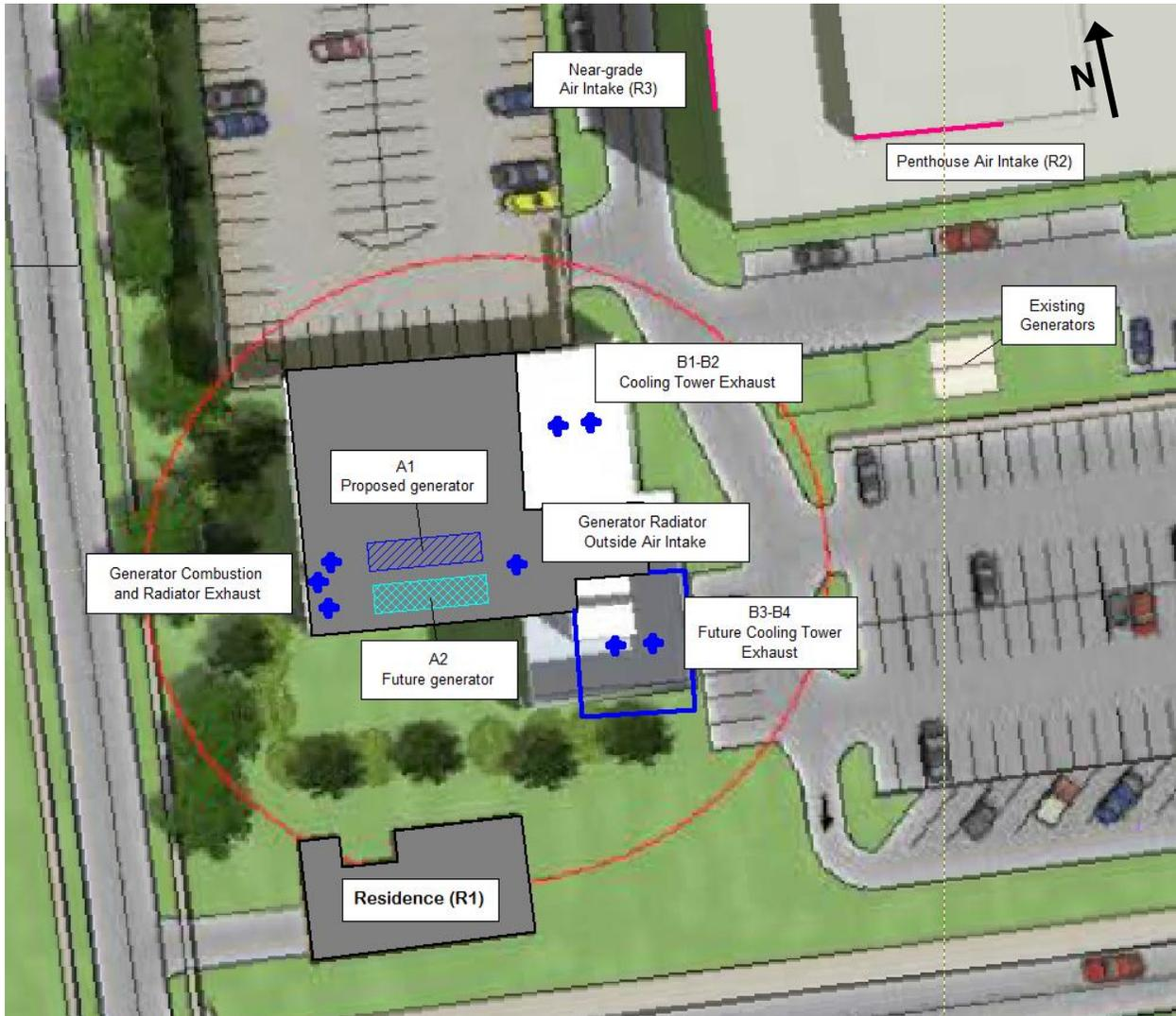
Figure 1: Plan Sketch of Equipment Layout for New Energy Plant
