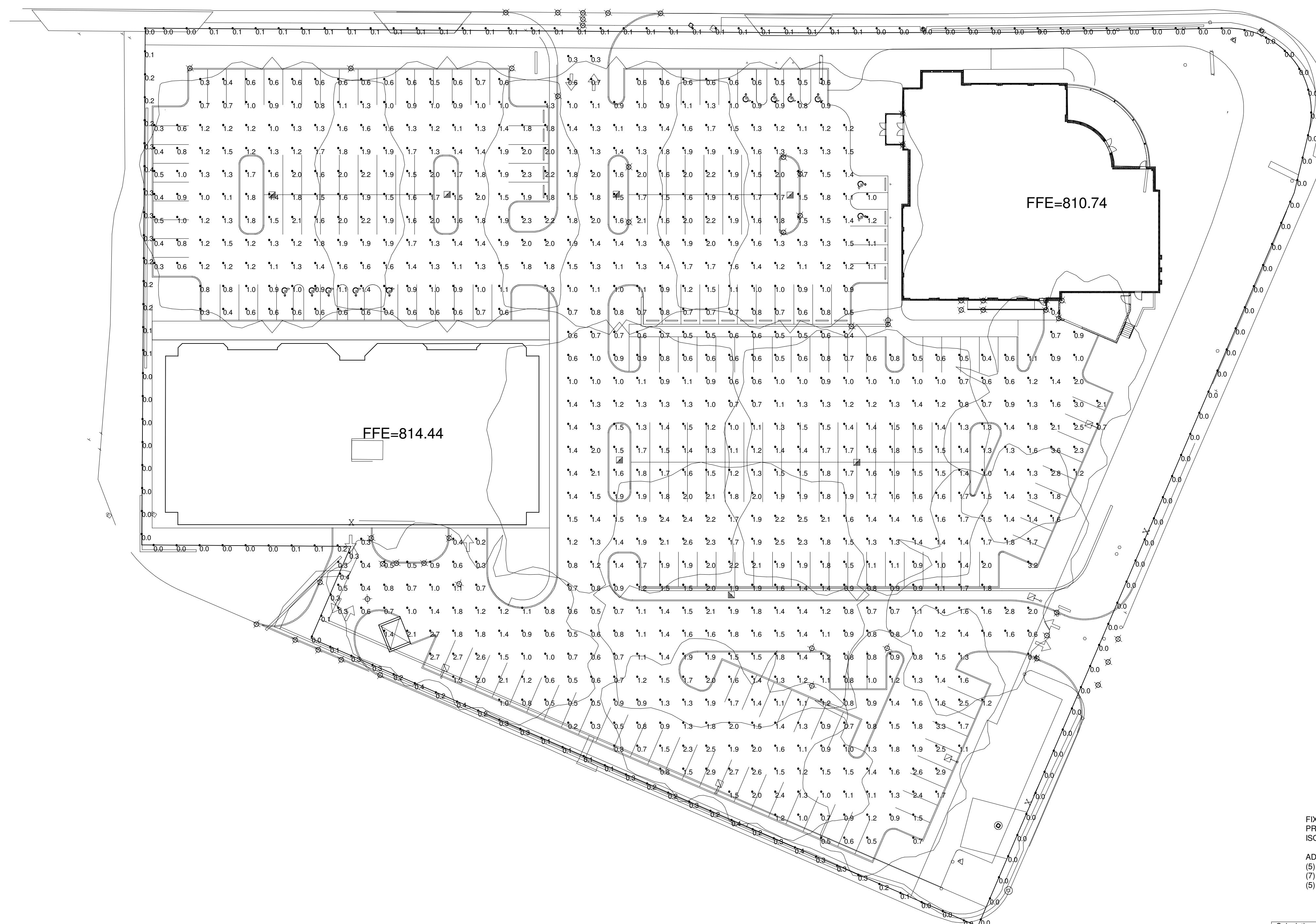
Fixture mounting height: 24' AFG (22' POLE + 2' BASE)
