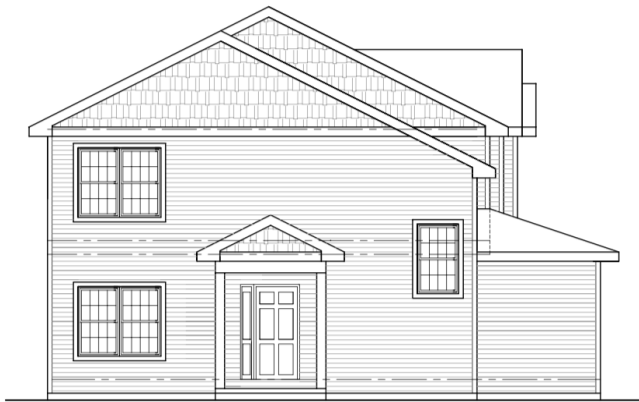
LEFT SIDE ELEVATION 1/4"=1'-0"
