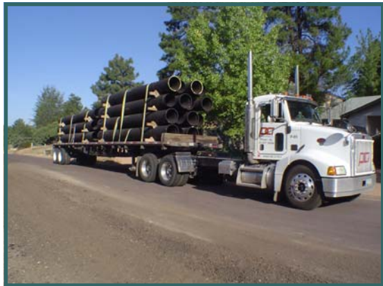
18” Ductile Iron Pipe for “Line B”
