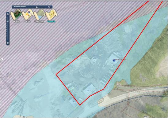
Flood Plain (blue Shading) hatched area is the river channel
