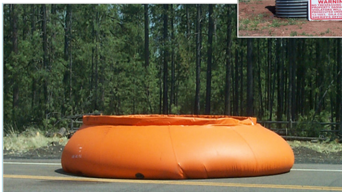
Water sources identified for Wildfire Protection (above) and "pumpkin tanks" (left) purchased by Gila County that can be set up close to a fire scene.
