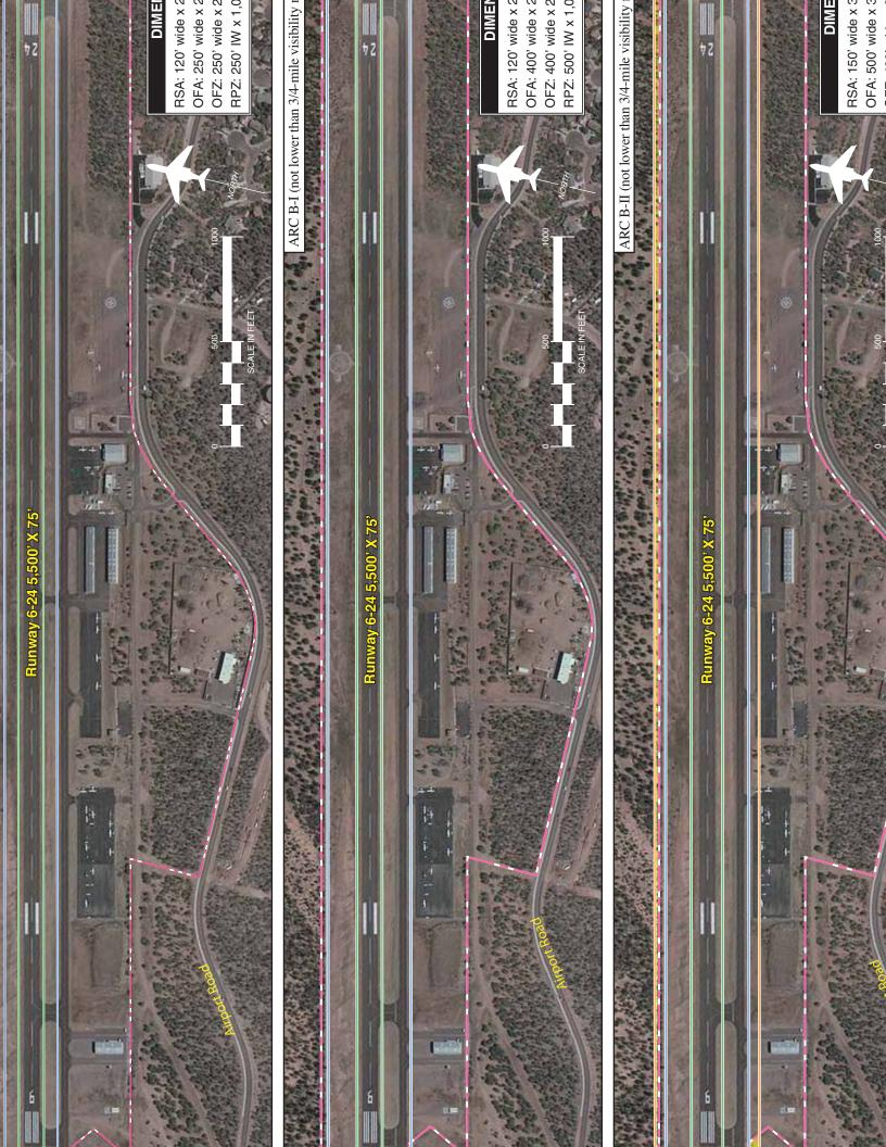
ing requirements. The bottom of **Exhibit 4B** depicts the safety areas when the airport progresses to ARC B-II design standards without other improvements being made. As depicted, the enlarged ARC B-II RSA would remain on airport property; however, the larger RSA would need to be improved to meet standards as described above, similar to the existing RSA requirements.
